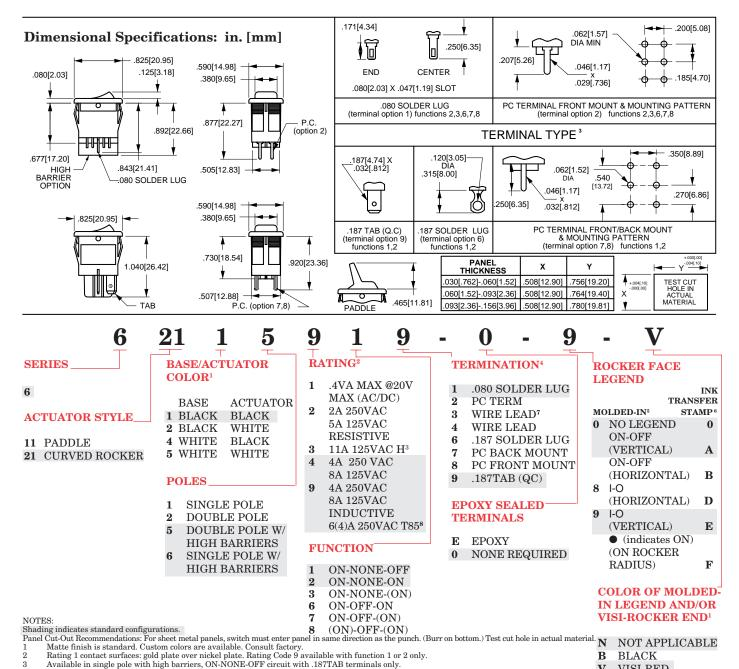
Terminations 1, 2 and 3 are not available with function 1. Terminations 4, 6, 7, 8 and 9 are available with function 1 or 2 only. Molded-in Legend available only with Visi-Rocker Option.
